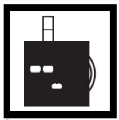
3. Insert the tube containing Indicator into the right-hand opening of the Color Comparator.
