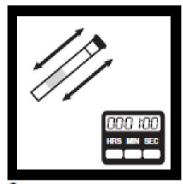
Stopper the tube and shake vigorously for exactly one minute. A pink color will develop if nitrite is present.
