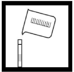
2. Fill the second viewing tube to the 5-mL mark with sample. This will be the prepared sample.
