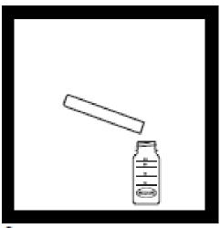
2. Pour the contents of the tube into the mixing bottle.
