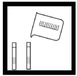
1. Thoroughly rinse two viewing tubes with sample and fill to the 5-mL marks.
