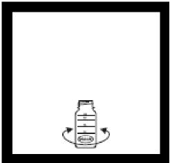
4. Swirl to mix. If the water remains colorless, the phenolphthalein alkalinity is zero. If it is, skip to step 7.
