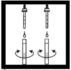
4. Add 3 drops of Nessler Reagent to each viewing tube and swirl to mix. Stopper both tubes.
