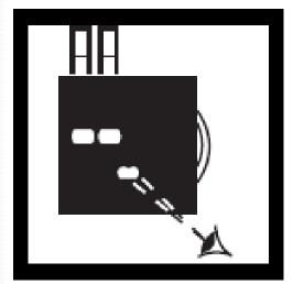
10. Read the mg/L nitrite-nitrogen (N) through the scale window.
