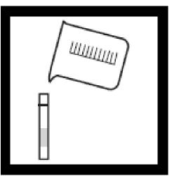
Fill another tube to the 5-mL mark with untreated sample.
