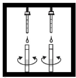
Add 1 drop of Rochelle Salt Solution to each viewing tube and swirl to mix.
