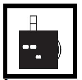
Place the tube into the right opening of the Color Comparator.
