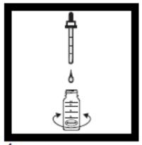
4. Add one or two drops of Hardness 2 Test Solution and swirl to mix.
