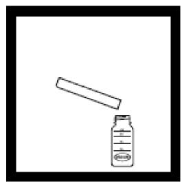
Pour the contents of the tube into the mixing bottle.
