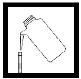
1. Fill one viewing tube to the 5-mL mark with deionized water. This will be the reagent blank.
