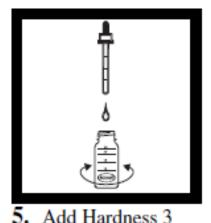
Titrant Reagent one drop at a time. Dispense the solution no faster than one drop per second. Do not allow the dropper to contact the side of the mixing bottle. Swirl the mixing bottle after each drop. Count each drop. Continue until the solution color changes from pink to blue.
