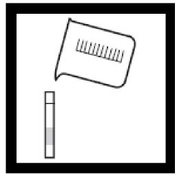
Rinse a viewing tube several times with sample, then fill to the 5-mL mark.
