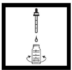
5. If the sample turns pink, add Sulfuric Acid Standard Solution one drop at a time. Count each drop. Swirl the mixing bottle after each drop. Add drops until the sample turns colorless.
